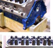
327cu in, maximum power 393bhp. Max torque occurs at 4500rpm [386ft lbs]. Torq exceeds 362ft lbs from 3-5500rpm. Good idle quality. Will pull like a train!
